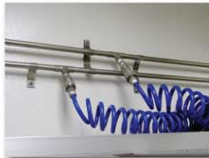
ReCIRC™ Through Rack requires inlet and outlet connections on rack
